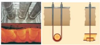
The maximum unsupported length above which supports (hangers) for radiant tubes are considered essential is given below:
