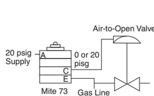
**Close an on-off valve in a gas line when line pressure drops below a set point.** Supply pressure at "A" is transmitted to valve from "C" when Mite is operating. When gas line pressure-monitored at "E"-drops below set point, trip occurs, and valve operator is vented to atmosphere.
