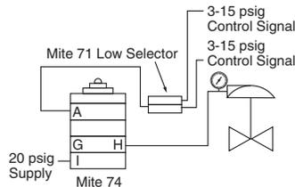
**Close an on-off valve when either of 2 signals drops to a set point.** Lower of 2 control signals is constantly fed to "A". Supply pressure at "I" is transmitted to valve "H" when Mite is operating. When trip occurs, valve is vented to atmosphere from "G".
