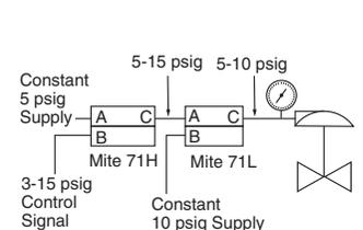
**Set 2 pneumatic pressure limits (high and low) within the range of a control signal, i.e., a double pneumatic stop.** Output from Mite 71H must stay within 5 to 15 psig when connected as shown. Output from Mite 71L to valve must stay within 5 to 10 psig.
