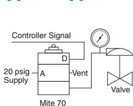
**Actuate an on-off valve when controller signal increases to set point.** Supply pressure at "A" is transmitted to valve from "B" when Mite is operating. When trip occurs, valve is vented to atmosphere.
