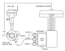
To adjust the cut-off set point, remove the cap and adjust the spring adjusting screw until desired outlet cut-off pressure is achieved. Turning the adjusting screw clock-wise will increase the cut-off setting and turning it counter-clock wise will reduce the cut-off setting. Note that the lock-up relay has a differential pressure of 2.5 psig (.17 BAR). Replace cap securely after having re-adjusted the cut-off set point.
